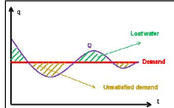
Different scenarios have been tested on the 24 kilometers canal benchmark (changes in the level references, variation in off-takes demand and heavy rain), showing a cost reduction of up to 25%, considering both lost water and unsatisfied demand.
